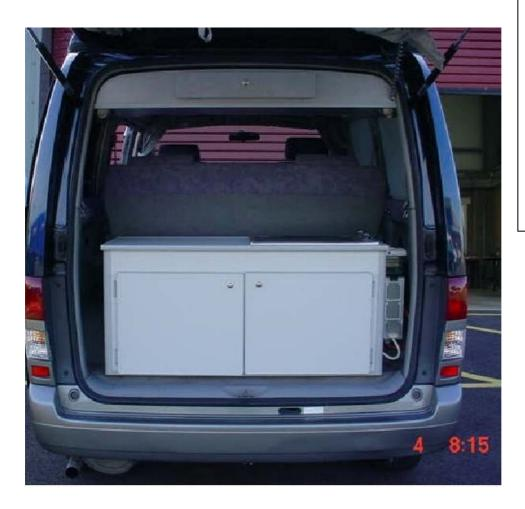
In this vehicle the kitchen facilities are fitted at the rear of the vehicle. The interior of the vehicle remains largely unaltered and does not provide living accommodation as would be found in a caravan.
