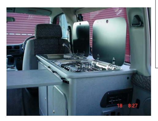
In this vehicle the kitchen facilities are fitted in the centre of the vehicle. The interior of the vehicle remains largely unaltered and does not provide living accommodation as would be found in a caravan.
