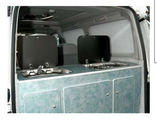
This vehicle is fitted at the rear with a kitchen unit. It may be accessible from inside or outside of the vehicle. Seats to the front of the unit may be forward or rearward facing or may be removed. The interior of the vehicle remains largely unaltered and does not provide living accommodation as would be found in a caravan. The vehicle is therefore primarily a passenger vehicle (sometimes termed a "Day Van" due to the facilities available) and is **not a motor** caravan
