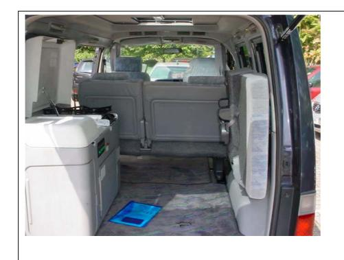
This example has a "kitchen facility" fitted in the rear of the vehicle. The interior of the vehicle remains largely unaltered other than a table may be fitted in front of the second row of seats. This vehicle is considered to be primarily a passenger vehicle and **not a motor caravan**.
